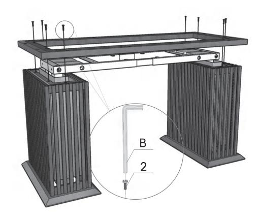
Raise the desktop base plate and lock the screws.
