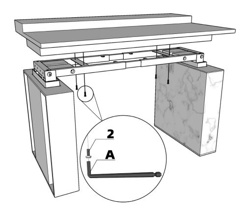
Cover the metal cover plate and lock the screws.
