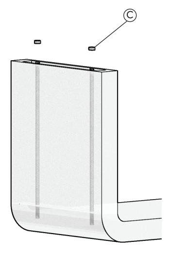
Fix the screw and gasket, and then put in 18mm nut.
